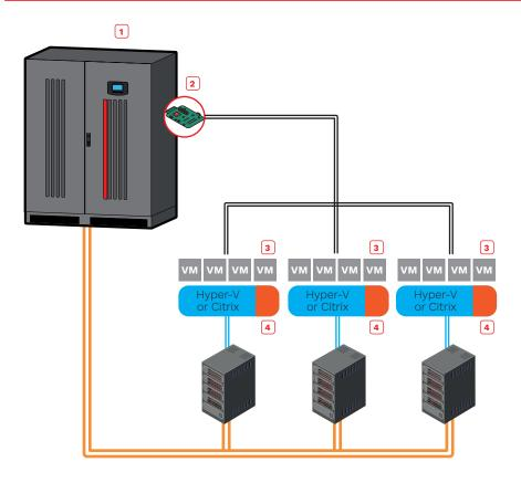
PowerShield<sup>3</sup> software should be used for managing setup with UPS, a specific script to shut down the virtualised system must be used, UPS must have a NetMan 208 board installed.
