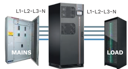
4-wire (L1-L2-L3-N) installation
