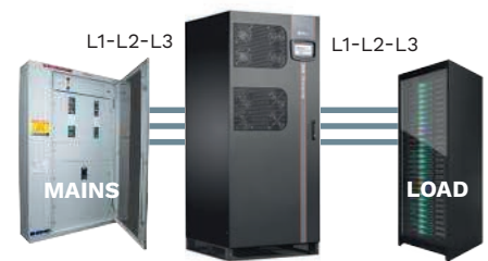
3-wire (L1-L2-L3) installation
